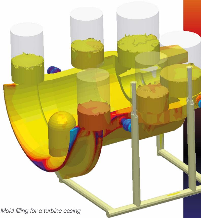
Mold filling for a turbine casing
