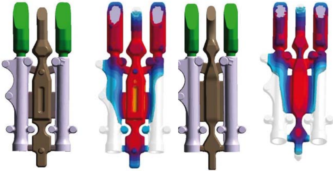
Fig. 9: Optimized gating system and permanent mold layout for an aluminum motorcycle fork (left: original gating layout and hotspot distribution, right: optimized gating layout with directional solidification [16]).
