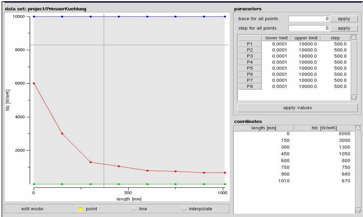
Fig. 1: Typical plot of heat transfers between a water cooled copper mould and a strand.
