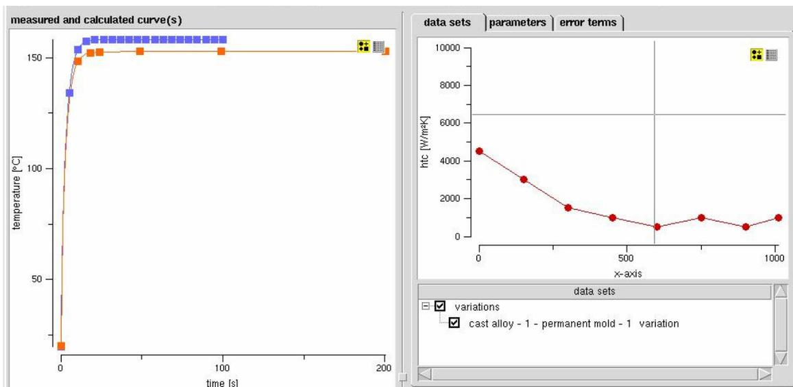
Fig. 2: The two temperature curves (left) are in a good agreement. The corresponding heat transfer coefficient is show on the right.
