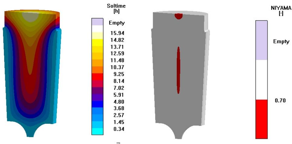
Fig. 7: Although the solidification is directional as indicated by the plot of the local solidification times (left), centre line shrinkage will appear due to insufficient risering. This can be detected with the Niyama criterion (right).
