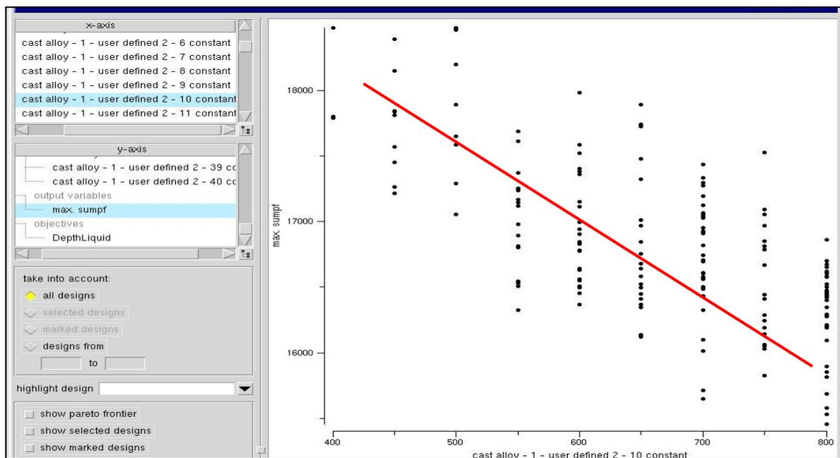
Fig. 4: Scatter chart for a water spray nozzle which belongs to the zone 3. On the x-coordinate the heat transfer coefficient  $[W/m^2K]$  of a spray nozzle is plotted and the y-coordinate shows the liquid pool depth  $[mm]$ . A clear tendency can be found.
