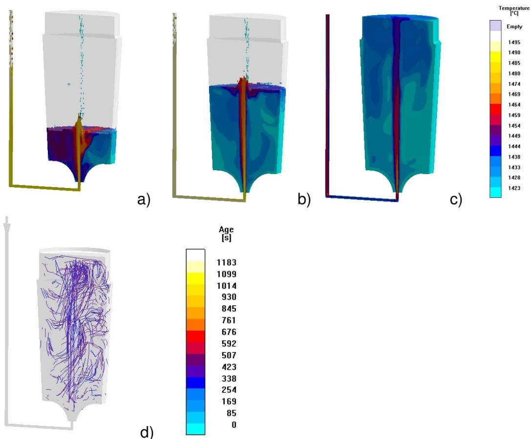
Fig. 6: Due to the quite simple shape of the bottom pouring system a fountain – like filling can be observed (a-c). The temperature loss during the filling process is quite low. The occurring turbulences are visualized by tracer particles (d).
