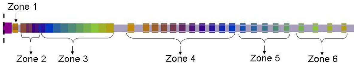
Fig. 3: The secondary cooling is partitioned into 6 different zones; the left picture shows the cooling zones in total.
