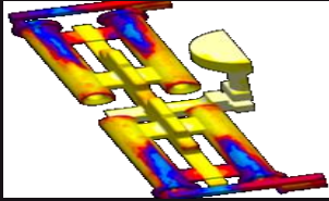
Under Riser Defects
